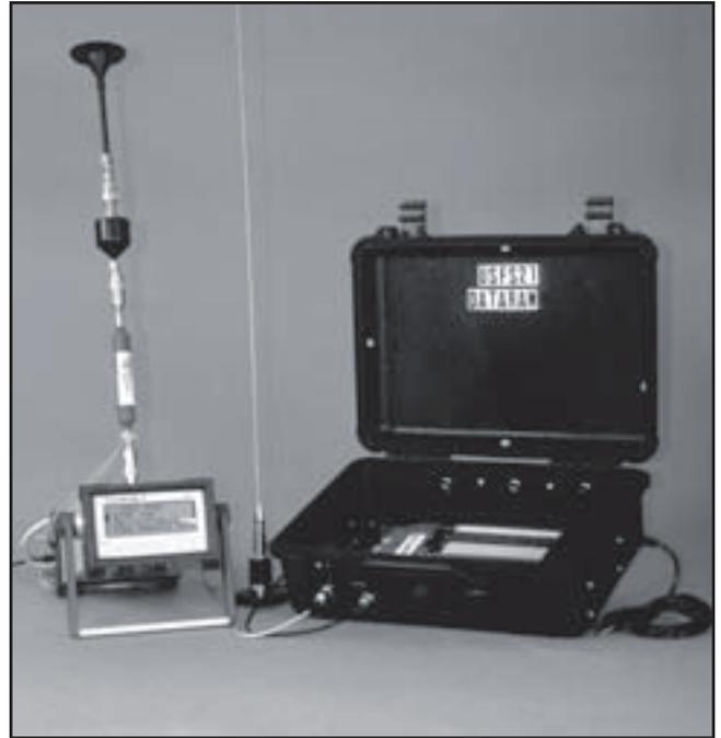
Figure 6—DataRAM4 connected to the telemetry unit.
