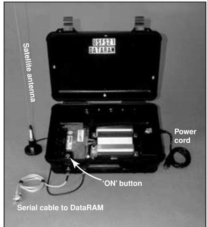
Figure 5—Remote telemetry unit used with the DataRAM4.
