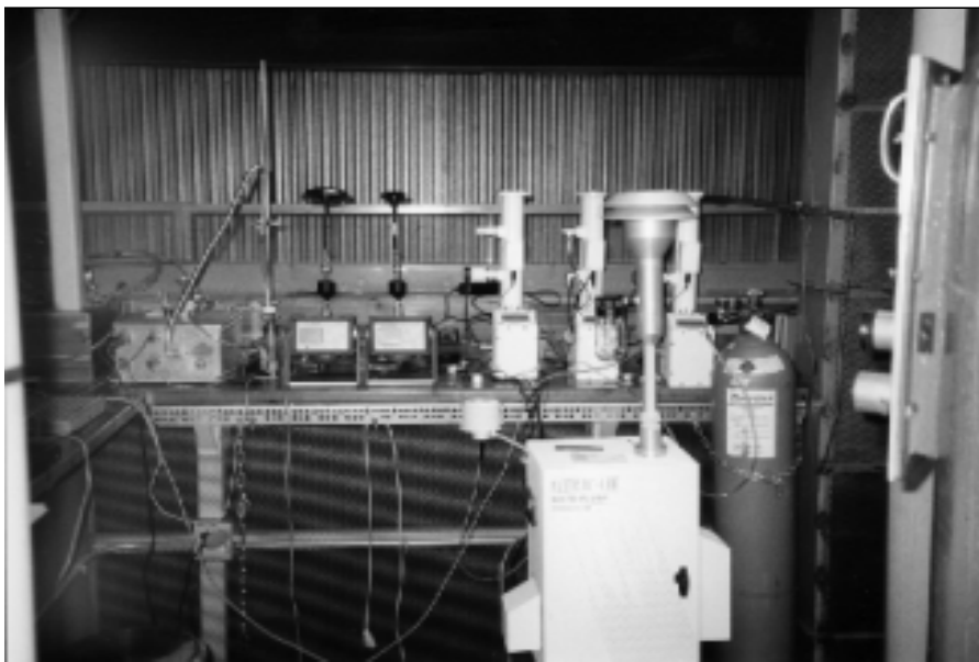
Figure 3—Instrument layout on the smoke platform in the burn chamber.
