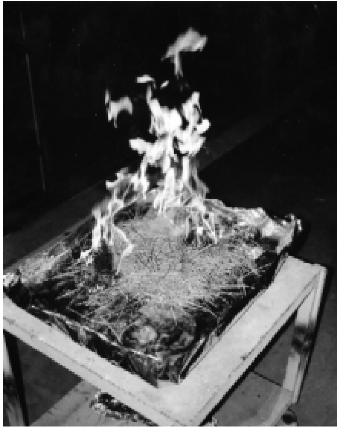
Figure 4—An example of the firebeds of pine needles used to produce smoke in the laboratory burn chamber.
